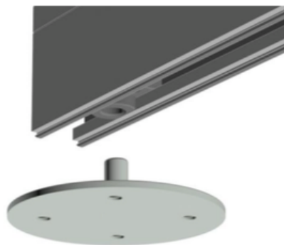
Picture 4.3: Installing pivot round flange
