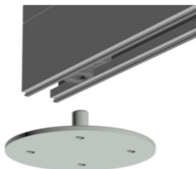
Picture 4.3: Installing pivot round flange
