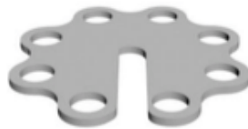
Picture 10.1: Special tool for adjusting the rollers
